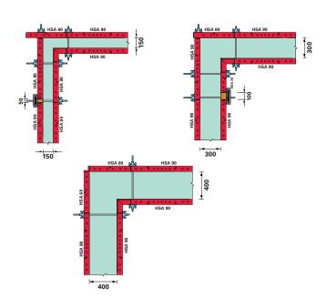
Columns with dimensions ranging from  $150 \times 150 \text{ mm}$  up to  $900 \times 900 \text{ mm}$  can be formed using 900 mm wide panel, without requiring any special panels.
