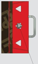
The triangular slot in panel has a three point of contact that ensures better rigidity and tightness when the wedge clip is locked into position.
