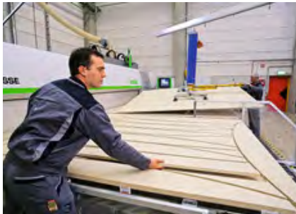
The CAD planning data is sent directly to the CNC machine. Here, individual panel cuts are created.
