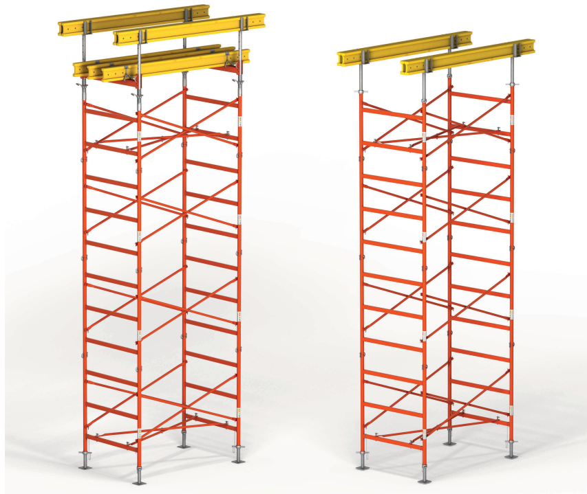
Load-bearing capacity of up to 55 kN per leg in accordance with DIN EN 12812 Basic dimensions: 1,25 m x 1,50 m / 1,25 m x 2,00 m / 1,25 m x 2,50 m Continuous height adjustment with only two frame sizes: 1,00 m / 1,50 m
